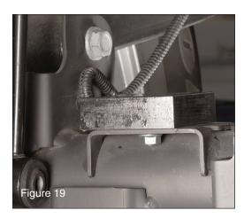
Install the bump stops to the axle pad with the 3/8" flat head screws and flange nuts using a 5.5mm hex key and tighten. (FIG 19).
