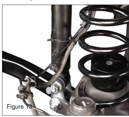
Loosely re-attach the lower shock to the new bracket using the original hardware and for 2011 and newer models zip tie the brake lines to the shock as shown. (FIG 13)
