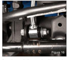
Loosely attach the sway bar links to the axle mount using the original hardware and 7/16" washers as shown. (FIG 16)
