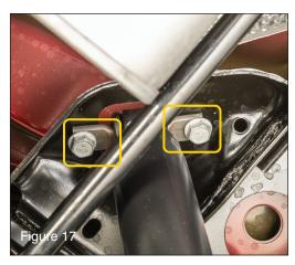
Raise rear end and properly support using jack stands. Disconnect the rear trackbar bracket from axle using 21mm socket and loosen the frame end mount, remove rear lower shock bolts and sway bar end links using a 18mm socket & open end wrench (FIG 17).
