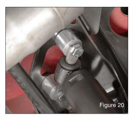
Install the original shocks with the provided spacers and M10 hardware and 3/8" washers using a 17mm socket. Torque to 37ft-lbs. (FIG 20)
