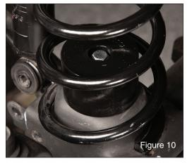
With axle in drop position, place bump stop in coil spring, and install coil springs. Attach bump stop to axle using the 3/8" hex head bolts, washer and flange nut, tighten using a 9/16" socket. Repeat this on other side of the vehicle. Raise axle just enough to keep the springs in place. (FIG 10)
