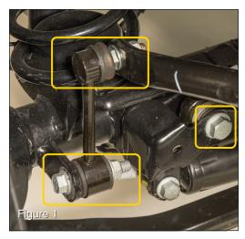
Remove the front sway bar end links from the axle mount using a 18mm socket and open end wrench, save hardware, then from the sway bar
