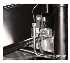
For 2007-2010 model years install the brake line brackets using the original hardware to the frame and tighten. Use the supplied M6 hardware, washer on the nut side, to attach brake line to the bracket and tighten. (FIG 12)
