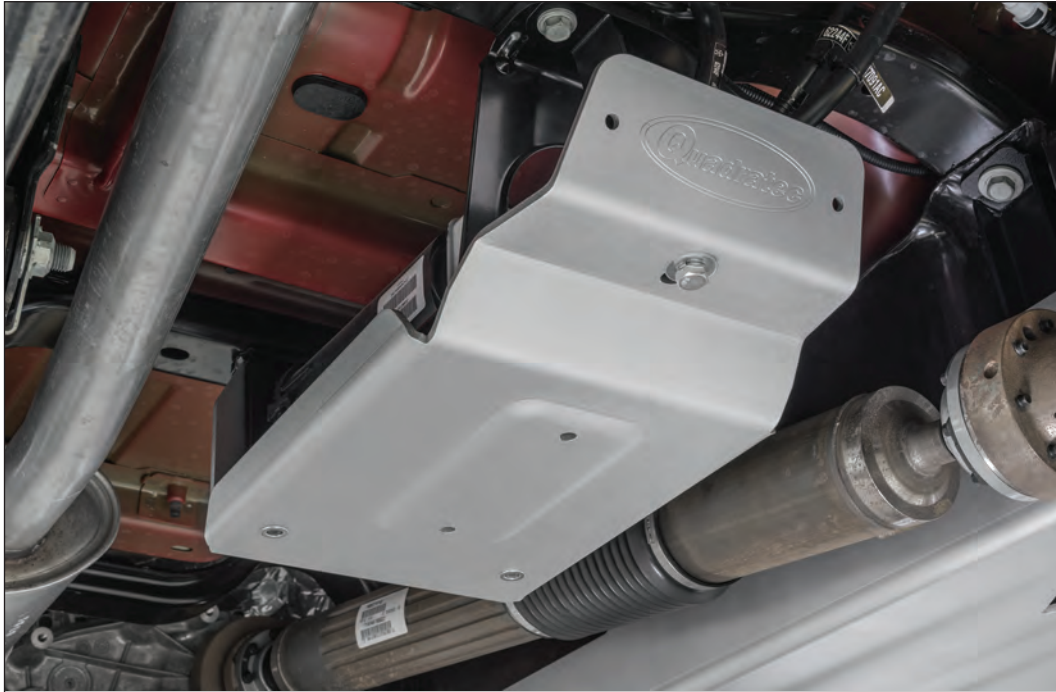
Evap Canister Skid Plate Installation Complete. View from Rear of vehicle.
