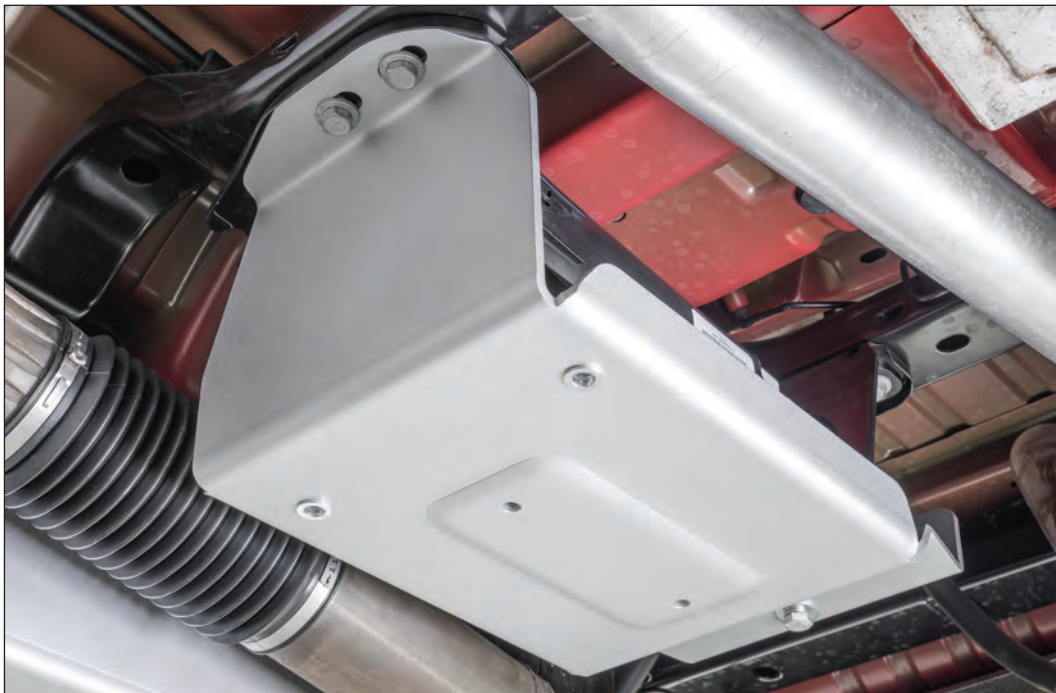
Evap Canister Skid Plate Installation Complete. Rear view of installed skid plate.
