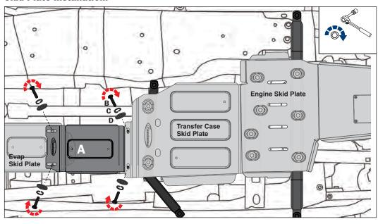
**STEP 1:** Put on safety glasses. With the Transfer Case and Evap Skid Plates installed, slip the rear Rear Transfer Case Skid Plate (A) under the back of the main Transfer Case skid and overtop of the Evap Canister skid plate.
