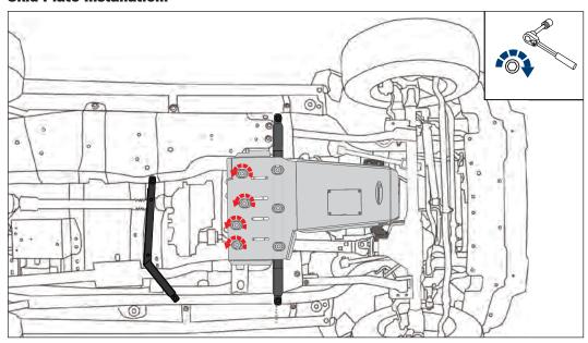
**STEP 3:** Loosen, but do not remove the rear fasteners of the Quadratec Engine Skid plate with a 17 and 19mm sockets. This allows room to mate the Transfer Case skid plate as shown below.
