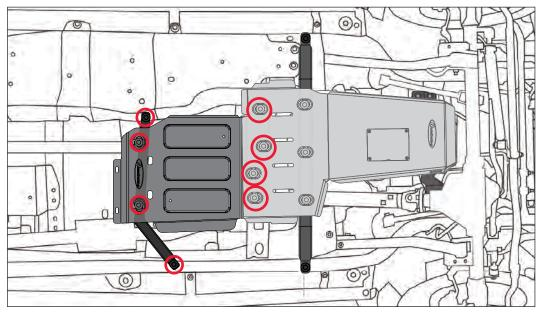
STEP 6: Make sure that all the skid plates align to your liking and then fully tighten all the fasteners. Using a torque wrench tighten all M10 bolts to 36 ft lbs and all M12/factory fasteners to 48 ft lbs.
