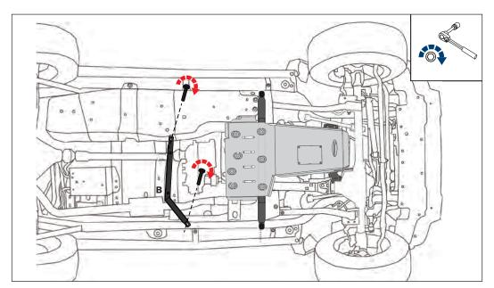
**STEP 2:** Using an 18mm socket Secure the new Cross Brace onto the frame using the factory transfer skid plate mounting locations and (2) factory fasteners. Snug but do not fully tighten the bolts at this time.
