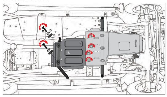
STEP 5: Install the (2) M10x30 bolts (C), lock washers (D) and flat washers (E) through the holes at the rear of the skid pate and thread them into the cross brace. Snug but do not fully tighten with a 17mm socket. Next, loosely tighten the rear bolts of the engine skid plate with a 17mm and 19mm socket.
