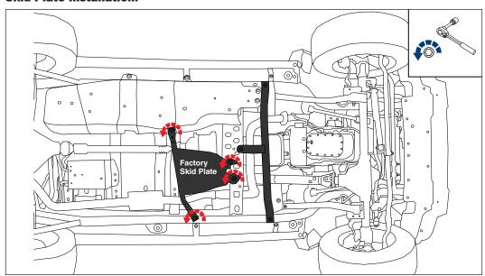
**STEP 1:** Put on safety glasses. Removal of the factory Transfer case skid plate: this step is also covered in the engine skid plate instructions. Remove the 4 factory bolts with a 18 mm socket. Discard the factory skid plate, it will not be reused.
