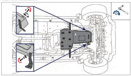
**STEP 7:** With help from a friend, lift the skid plate (A) into place and attach the front of the skid plate to the mounting brackets (B&C) with (2) M10x30 bolts (F), lock washers (L) & flat washers (M). Snug the bolts with a 17mm socket, not fully tight.
