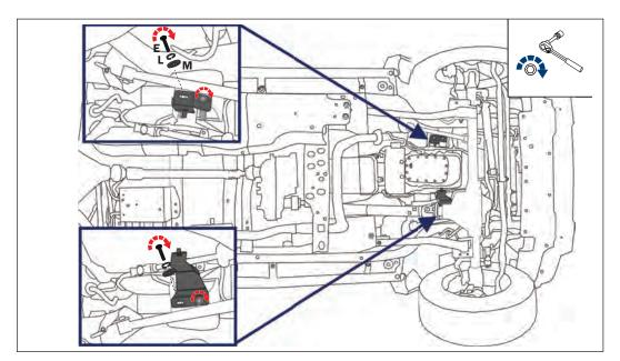
**STEP 4:** Install the other (2) M10x20 Bolts (E), lock washers (L), and flat washers (M) into the rear slot of the mounting brackets and hand tighten the bolts into the nut plates (J). Snug but do not fully tighten all the M10x20 bolts with a 17mm socket.
