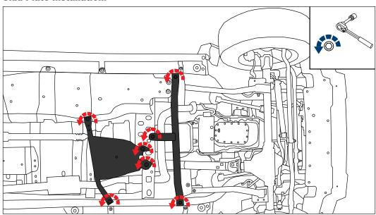
**STEP 1:** Put on safety glasses. Locate the Factory Transmission Cross brace (automatic only) and the Factory Transfer case skid plate. Remove the factory fasteners with a 18mm socket. The cross brace and transfer case skid will not be reused.
