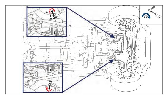
**STEP 2:** Locate the engine frame ears where the engine attaches to the frame. Slide the (4) M10 Nut Plates (J) inside the frame ears so that the threaded hole aligns with the holes in the frame. Finger tighten (2) M10x20 bolts (E), M10 lock washers (L), and M10 flat washers (M) into the front hole on either side.
