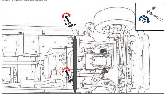
**STEP 5:** Install the Cross Brace (D) into existing holes in vehicle frame with (2) M12 bolts (H), lock washers (N), and large diameter flat washers (P). Snug but do not tighten the bolts with a 19mm socket to allow for alignment before final tightening.
