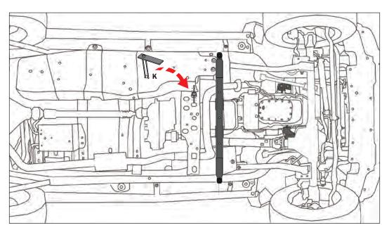
**STEP 6:** Install the Long M10 nut plate - with wire fish (K) inside the vehicle's transmission cross member so that the threaded hole aligns with the rightmost hole in the cross member.
