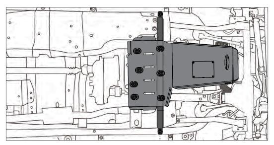
STEP 10: Make sure everything aligns to your liking before fully tightening the bolts. Start tightening the bolts from front to back. Tighten all M10 bolts with 17mm socket and a torque wrench to 36 ft lbs. Tighten all the M12 bolts with a 19mm socket and a torque wrench to 48 ft lbs.
