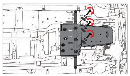
**STEP 8:** Install (3) M10x30 bolts (F) with lock washer (L), and flat washer (M) into the front 3 holes in the skid plate and thread them into the cross brace. Snug but do not tighten.
