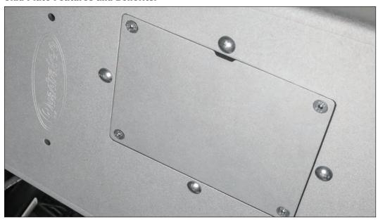
This skid plate has been thoughtfully designed to allow access for engine oil changes. In order to access your drain plug, remove the 4 countersunk hex head bolts with a 4mm hex key and remove the panel.
