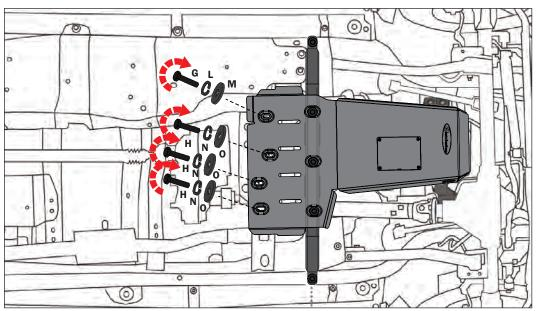
STEP 9: Next, install the (1)M10x40 bolt (G), lock washer (L) and flat washer (M) right rear hole of the skid plate and thread it into the long M10x30 nut plate (K) that was previously installed in the transmission cross member. Install the (3) M12x40 bolts (H), lock washers (N), and small diameter M12 flat washers (O) into the remaining rear holes of the skid plate. Snug but do not tighten.
