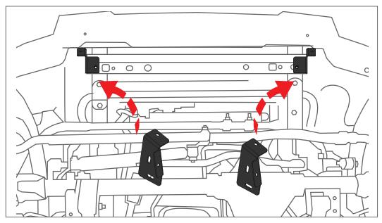
**STEP 2:** Position the Left and Right Mounting brackets (B) against the front crossmember of the vehicle as shown.
