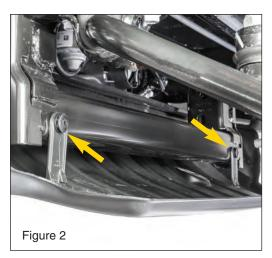
Next, remove the two plastic push rivets on the backside. (FIG2) Remove the splash guard. Note: This will not be reused with your Quadratec skid plate.
