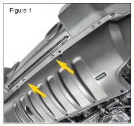
**STEP 1:** Put on safety glasses. Start by removing the factory splash guard. Remove the 4 plastic push rivets on the underside of the bumper. (FIG1)
