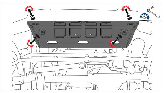
**STEP 4:** Place the Skid Plate (A) into place over top of the brackets (B) and secure with (4) M10 bolts, lock washers, and flat washers (C,D,E). Make the proper adjustments to align the skid plate to your liking and tighten all fasteners with a 17mm socket. Using a torque wrench, tighten all bolts to 36 ft lbs.
