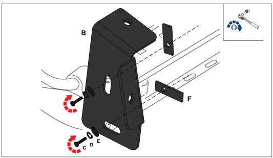
**STEP 3:** Secure the bracket (B) to the vehicle crossmember by inserting the (2) M10 Nut Plates (F) inside the frame and threading the (2) M10 bolts (C) through the brackets (B) along with (2) lock washers (D) and (2) flat washers (E) as shown. Repeat on opposite side of vehicle. Do not fully tighten bolts at this point. Some adjustment may be needed before final tightening.
