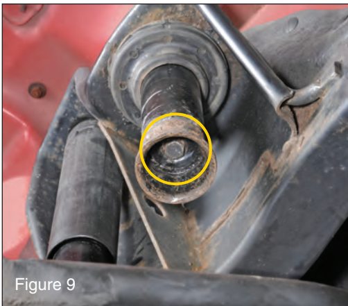
Figure 9 Remove bump stop cup using a 15mm socket (see FIG 9)
