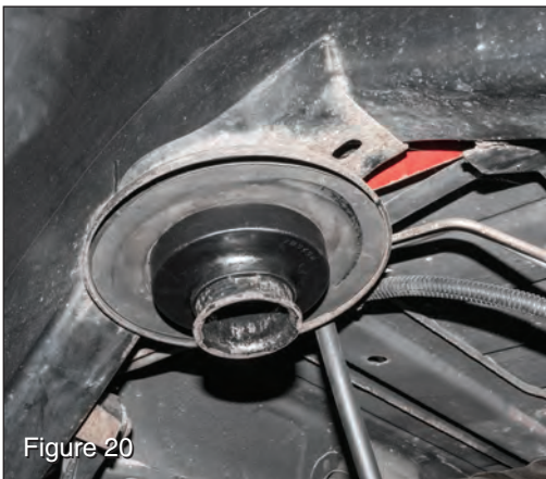
Install included coil spring spacer and secure using original bump stop cup and bolt (see FIG 20).
