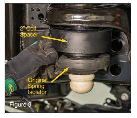
Remove factory coil spring isolator and place provided 2" coil spacer on top of Original Equipment spring isolator, exactly as shown (see FIG 9). Locate the new front bump stop in the kit.
