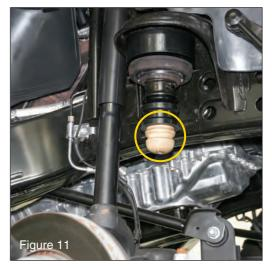
Install the original bump stop into the provided bump stop extension. (FIG 11). Repeat this on other side of the vehicle.
