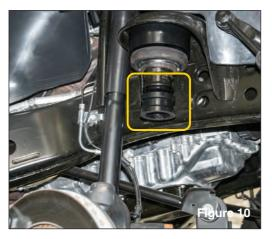
Remove original bump stop by pulling downward and twisting. Lubricate the provided bump stop spacer with dish soap and press it into the original bump stop cup. (FIG 10)
