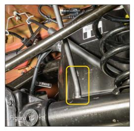
Disconnect axle housing vent line (FIG 15) Lower axle down and remove factory rear coil springs. Install new 3/4" coil spacer on top of the original equipment spring isolator (see FIG 16). Repeat on other side of vehicle.
