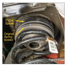
coil spacers. Re-attach brake line bracket to frame. Re-attach rear sway bar end links to axle housing using factory hardware and torque 60 ft lbs. Using factory hardware, re-attach bottom end of shock and torque to 56 ft lbs. Install wheels/tires and torque to 105 ft lbs. Finally, remove jack stands and lower vehicle onto the ground. Then, re-attach track bar using factory hardware and torque to 111 ft lbs.
