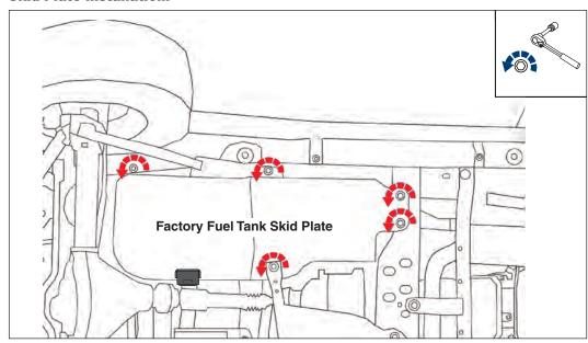
**STEP 3:** This step requires the help of a friend. Support the fuel tank and carefully remove the remaining 5 factory fuel tank skid plate bolts with a 18mm socket.
