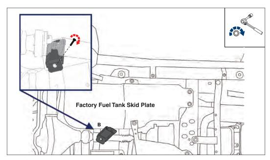
**STEP 2:** Place the mounting bracket (B) in place against the factory skid plate and reinstall the factory bolt through the mounting bracket. Snug but do not fully tighten.
