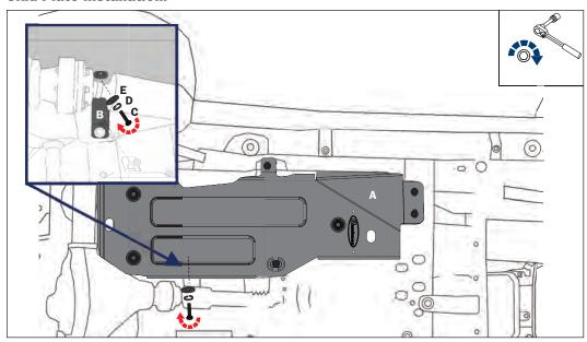
**STEP 5:** Now secure the skid plate (A) to the mounting bracket (B) by installing the M10x30 bolt (C), lock washer (D) and flat washer (E) through the skid plate and threading into the mounting bracket. Snug, but do not fully tighten with a 17mm socket.
