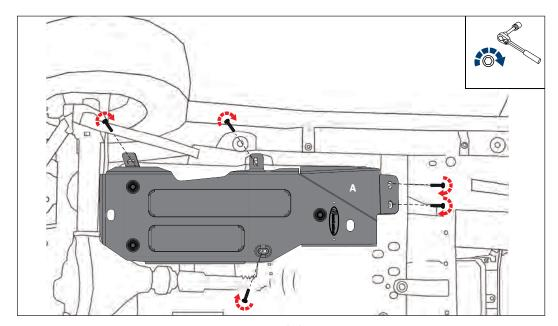
**STEP 4:** Slip the new Aluminum skid plate (A) overtop of your factory skid plate as shown. Reinstall the 5 factory bolts with a 18mm socket and ratchet. Gradually start each bolt and evenly draw the new skid plate into place in stages.
