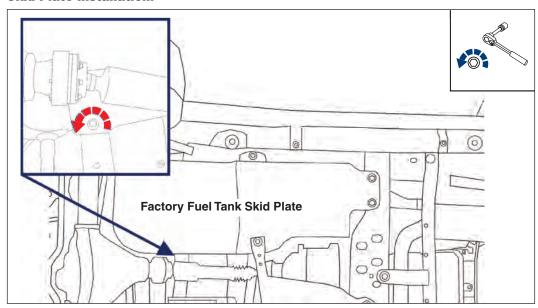
**STEP 1:** Put on safety glasses. Before you begin, make sure the fuel level in your tank is as low as possible. Locate the factory fuel tank skid plate. Locate and remove the Rear inboard factory mounting bolt with a 18mm socket.
