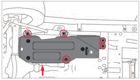
**STEP 6:** After the skid plate is fully installed tighten all factory bolts to 48 ft lbs with a torque wrench and a 18mm socket. Torque the M10x30 bolt (C) to 36ftlbs using a 17mm socket.
