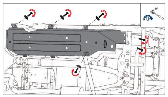
**STEP 4:** Slip the new Aluminum skid plate (A) overtop of your factory skid plate as shown. Reinstall the (6) factory bolts with a 18mm socket and ratchet. Gradually start each bolt and evenly draw the new skid plate into place in stages.
