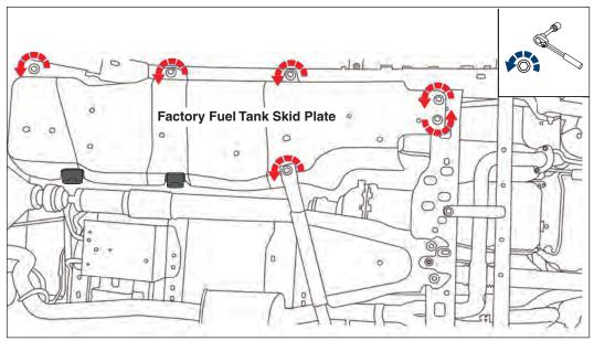
**STEP 3:** This step requires the help of a friend. Support the fuel tank and carefully remove the remaining (6) factory fuel tank skid plate bolts with a 18mm socket.
