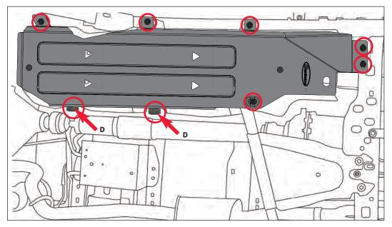
**STEP 6:** After the skid plate is fully installed tighten all factory bolts to 48 ft lbs with a torque wrench and a 18mm socket. Also, torque the (2) M10x30 bolts (D) to 36 ft lbs using a 17mm socket.
