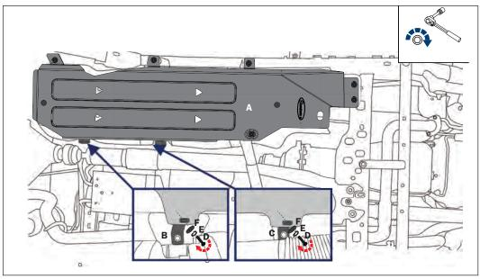
**STEP 5:** Now secure the skid plate (A) to the mounting brackets (B&C) by installing the (2) M10x30 bolts (D), lock washers (E), and flat washers (F) through the skid plate and threading into the mounting brackets. Snug but do not fully tighten the bolts with a 17mm socket.
