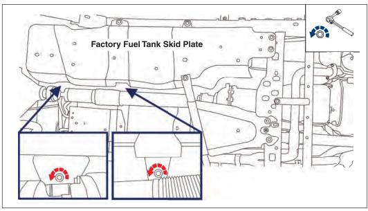
**STEP 1:** Put on safety glasses. Before you begin, make sure the fuel level in your tank is as low as possible. Locate the factory fuel tank skid plate. Locate and remove the (2) Rear inboard factory mounting bolts with a 18mm socket.
