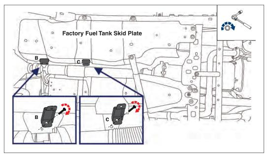
**STEP 2:** Place the Longer mounting bracket (B) against the factory skid plate at the rear of the tank and place the shorter (C) front mounting bracket in the forward location. Reinstall the factory bolts through the mounting brackets. Snug but do not fully tighten with an 18mm socket.
