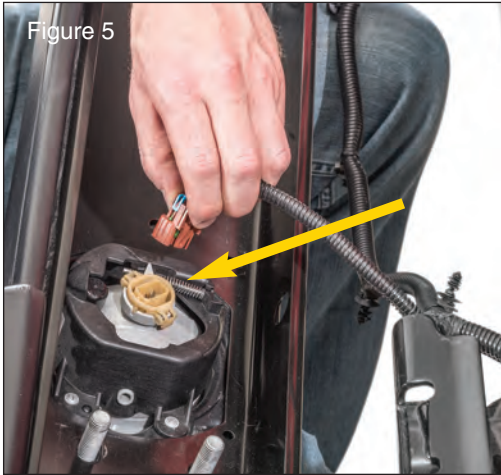
Disconnect the factory wiring harness from the bumper mounted fog lights. (FIG5)
