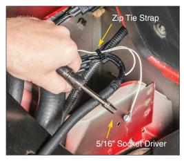
drill through the sheet metal as shown. Be careful to avoid over-penetrating and damaging the exterior of the vehicle body! Use a 5/16" socket driver or wrench to tighten the sheet metal ground strap screw. Use a zip tie strap to attach trailer harness to car harness.
