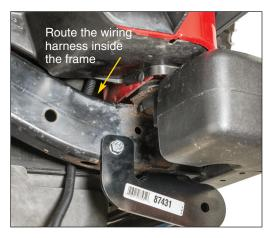
With all circuits connected, test ALL vehicle lamps to ensure that they are properly functioning and also test your trailer lamps.
