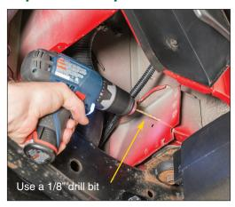
IMPORTANT! In order for the vehicle's tail lamps and the trailer lamps to function properly, a clean and secure electrical ground must be established for the trailer harness. Locate the approximate drill point as illustrated in the photo above. Using an 1/8" drill bit, carefully
