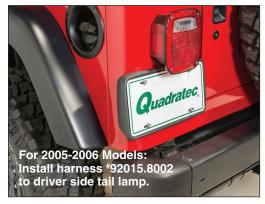
These instructions have been illustrated at the driver side lamp for '05-'06 applications. Installation for '98-'04 models takes place at the passenger side tail lamp but the procedures are identical.
