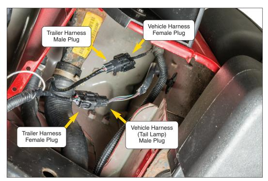
**Step 3: Connecting Hitch Wiring Harness**
