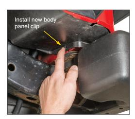
Route the Trailer Hitch Harness inside the frame rail and install the new body panel clip to secure the inner fender well liner.
