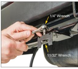
Find a suitable mounting location for the trailer hitch plug bracket. This should be approximately 6" from the receiver hitch tube. Some hitches provide a suitable mounting tab to attach the plug bracket. CAUTION: If drilling is required to install the plug bracket, use a 3/16" drill bit and be mindful of the gas tank, fuel lines and hoses along with
