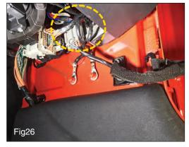
Now locate the harness back under the dash and install the "Christmas tree connectors" on the adapter harness back into the factory mounting holes. Secure all wiring out of the way with the supplied zip ties as shown in FIG26.
