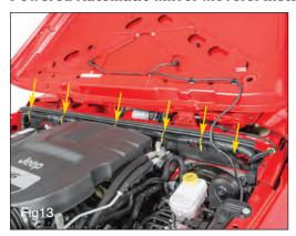
Route the Passenger harness along the factory loom at the back of the firewall as shown in FIG 13 and secure with the supplied cable ties. Next, route the drivers' harness to the hole in the firewall as
