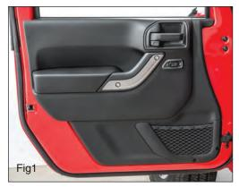
Put on safety glasses. In order to install your Quadratec Powered Automatic Mirror Movers you will need to remove your factory power mirrors. Start by opening your Jeep's driver's side door. Locate the inner door panel. You will need to remove this panel in order to disconnect your factory mirrors. Please consult our website for detailed instruction on door panel removal.
