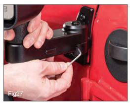
In the event you choose to remove your doors, there is a convenient block-open feature built into these mirrors. Swing the mirror out and locate small hole on the lower hinge assembly.
