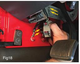
Locate the other end of the harness and remove it from its mounting location by pulling the "Christmas tree clips" free of the mounting holes. See FIG18.
