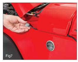
Pull the wire all the way under the cowl and under the hood. Leave just enough harness exposed to allow for installation of the mirror mover. (Fig7) Reinstall the factory hinge plate using the factory screws in the upper 4 holes. Snug using the supplied T40 Torx wrench. (Fig8)
