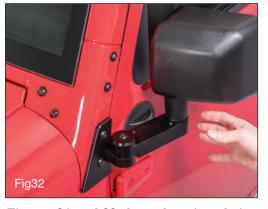
Figures 31 and 32 show the mirror being pulled away and automatically returning to its resting position.
