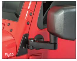
wrench gently snug the through bolt (Fig29) until the mirror does not return freely to it's resting position. Fig30 shows the mirror in the no-return
