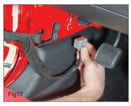
Disconnect the factory door harness connector from underneath the dash in the left of the driver's footwell as shown in FIG17.
