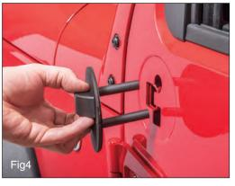
not be re-used. Reinstall the door panel. Locate the filler plate with bumper as shown in FIG4. The longer extension tube goes into the bottom hole on the door. Insert through door into the stock mirror location. Reinstall T40 Mirror Bolts into filler plate and tighten.
