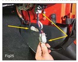
Install the supplied adapter harness between the factory connectors as shown and connect the Passenger's side mirror mover harness as shown in FIG25.
