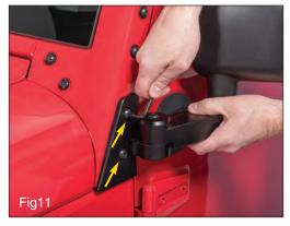
Tip the assembly into place and tighten the Torx bolts using the supplied T40 Torx wrench. Pull the excess harness wire from under the cowl so that it is not visible under the hinge plate or Mirror Mover Bracket. Repeat Mirror mover installation steps on the passenger side.
