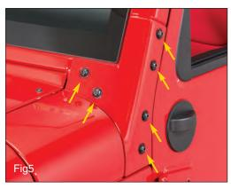
Locate the 6 T40 Torx bolts that hold on the windshield hinge plate. Remove all 6 bolts with supplied T40 Torx wrench. Carefully remove the hinge plate and set aside. Locate the Driver's Side Powered Mirror Mover with Wiring Harness.
