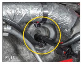
Pass the new wires through the slit in the grommet. Reinstall the grommet in the firewall. (FIG16)
