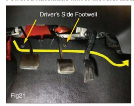
Now route the passenger side mirror mover harness from the driver's side footwell over to the passenger side footwell. (Fig21) Remove carpet retaining clips and pass the harness behind the carpet and underneath the retaining studs. Continue to route the harness
