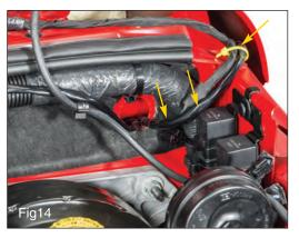
shown in FIG14 and secure with a supplied cable tie. Pass both the connectors and harnesses through the hole in the firewall and down into the drivers foot well.
