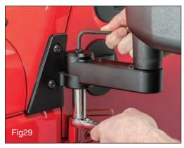
If your mirror is not returning properly to the fully closed position, pull the Mirror mover away from the vehicle. Using a 6mm hex key and a 17mm socket
