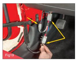
Install the supplied adapter harness between the factory connectors as shown and connect the Drivers side mirror mover harness as shown in FIG19.
