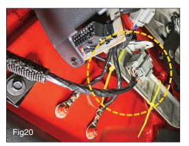
Locate the harness back under the dash and install the "Christmas tree connectors" on the adapter harness back into the factory mounting holes. Secure all wiring out of the way with the supplied zip ties. Take special care not to interfere with operation of any of the vehicle pedals or controls.
