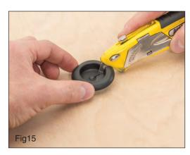
Slit the factory grommet with a razor knife as shown.
