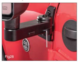
The 3mm hex key acts as a pin to hold the upper hinge in place. Gently allow mirror to return and contact the hex key as shown in FIG28. With the mirrors blocked out of the way, the doors can be removed without interference.
