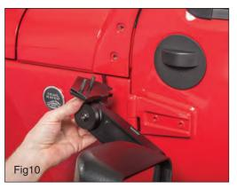
Place the two remaining factory screws through the mounting holes in the mirror mover and place the gasket on the backside of the mounting bracket as shown.
