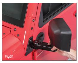
position. Next, back off the nut on the through-bolt slightly (approximately ¼ turn) until the mirror automatically returns freely and smoothly to its resting position.
