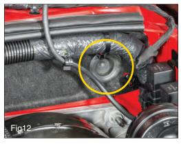
Wire harness routing and installation: Locate and remove the factory grommet shown in FIG12. Both the driver and passenger harnesses will pass through this hole in the firewall. Note: Factory Hardtop models use this grommet for rear washer fluid hose.
