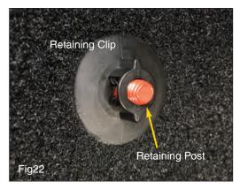
under the carpet and behind the center console. Reinstall the factory carpet and the carpet retaining clips (Fig22). DO NOT allow wiring harness or carpet to interfere with operation of pedals. Such interference could cause loss of vehicle control.
