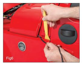
You will now need to route the attached wire harness and connector behind vehicle's cowl as shown (Fig6). Due to manufacturing tolerances you may need to gently pry the panel gap apart using a non-marring pry tool or a flat blade screwdriver wrapped in tape.
