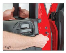
Locate Two T40 Torx bolts on the inside door panel. Remove bolts with the supplied Torx wrench. Take care to support the mirror on the outside of door to prevent damaging factory mirror. Remove mirror. Retain factory bolts for installation of filler plates. Factory mirrors will
