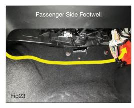
Continue routing the wires behind the carpet and under the retaining posts in the passenger footwell as shown in FIG23.
