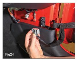
Disconnect the passenger side Factory door connector. Locate the other end of the harness & remove it from its mounting location by pulling the "Christmas tree clips" free of the mounting holes.
