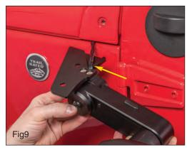
Route the harness wire in the machined recess of the mirror mover before installation as shown.
