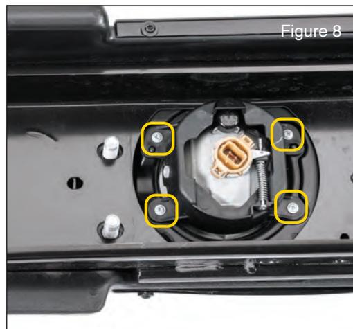
*Now remove the factory fog lights from the factory bumper with a phillips screwdriver. (FIG8) Save factory fog lights for installation into the new QRC Bumper.*
