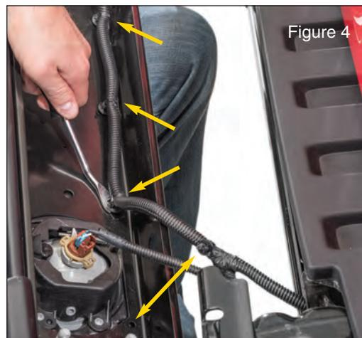
Be careful not to damage the fog light harness. Use a forked pry tool to remove the harness retaining clips from the backside of the bumper. (FIG4)
