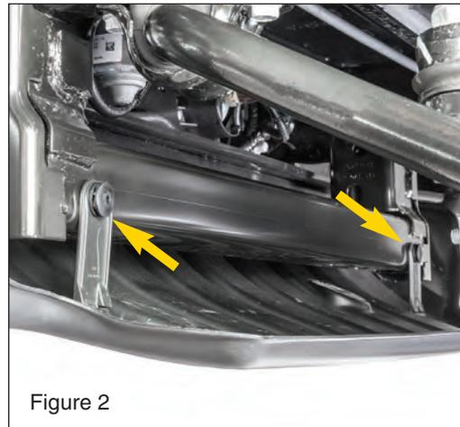
Next, remove the two plastic push rivets on the backside. (FIG2) Remove the splash guard. Note: This will not be reused with your Quadratec bumper.
