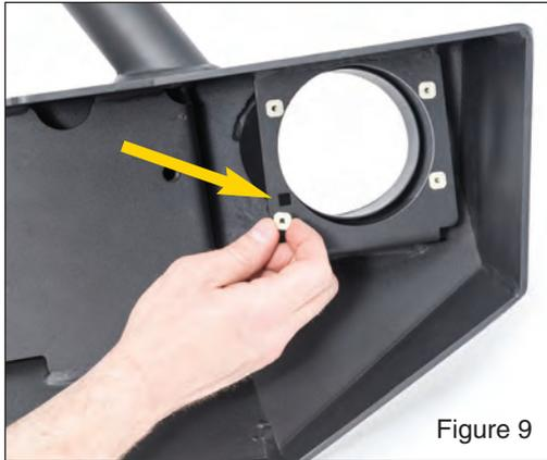
On the new bumper, install 4 plastic push nuts into the square holes on the backside of each foglight mount housing. (FIG9)
