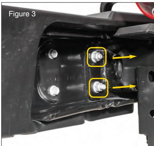
Next remove the factory bumper. Using an 18mm socket remove the 8 bumper retaining bolts. There are 2 on the inside and outside of each frame rail. (FIG3) Carefully remove the bumper from the frame rails.
