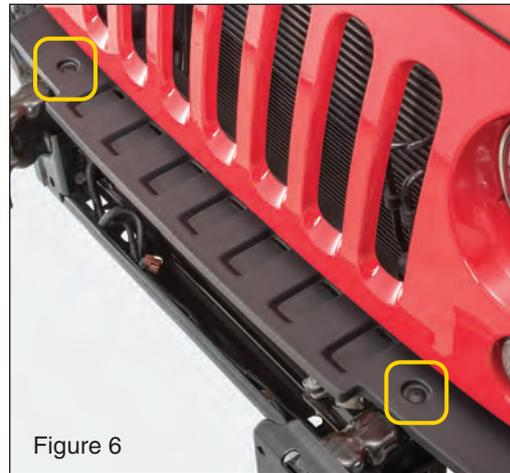
*Next, remove the Factory frame guard. Locate the plastic screw rivets on either side. (FIG6)*
