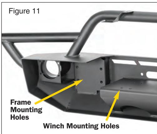
*Before installing the bumper you must first install your winch and fairlead into the bumper according to your winch installation instructions.*
