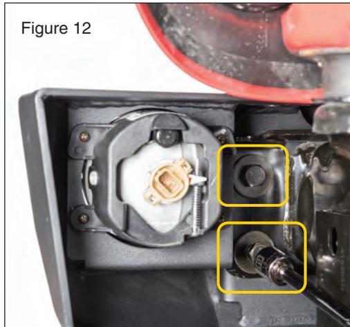
Secure the bumper to the Frame with the supplied M12 bolts, lock washers and flat washers using an 18mm socket and ratchet. Torque the bolts to 66ft pounds. (FIG12)
