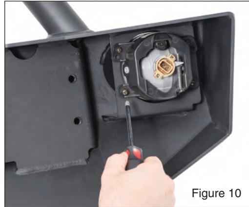
Place the factory Fog lights in place and secure them with the 8 provided Phillips head screws and a Phillips screwdriver. (FIG10)
