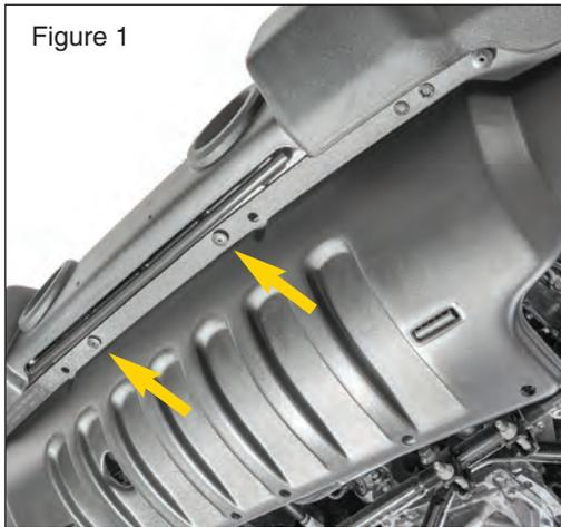
Put on safety glasses. Start by removing the factory splash guard. Remove the 4 plastic push rivets on the underside of the bumper. (FIG1)
