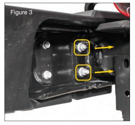
Next remove the factory bumper. Using an 18mm socket remove the 8 bumper retaining bolts. There are 2 on the inside and outside of each frame rail. (FIG3) Carefully remove the bumper from the frame rails.
