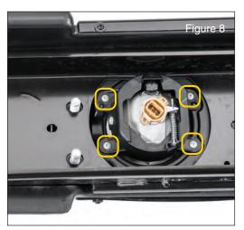
Now remove the factory fog lights from the factory bumper with a phillips screwdriver. (FIG8) Save factory fog lights for installation into the new ORC Bumper.
