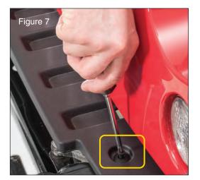
Remove the plastic screw rivets with a phillips screwdriver. (FIG7)
