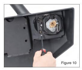
Place the factory Fog lights in place and secure them with the 8 provided phillips head screws and a phillips screwdriver. (FIG10)
