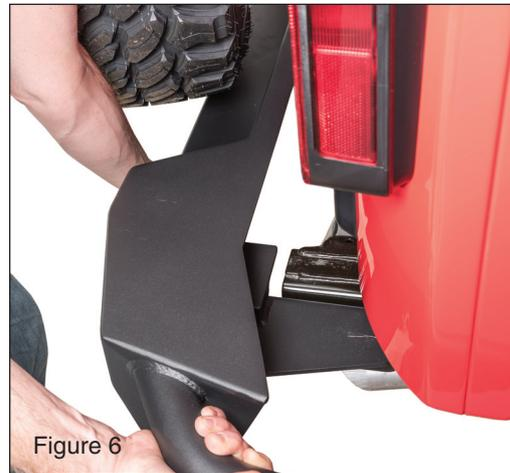
*person, and with the tailgate partially open lift the bumper and gently rest it on the frame rails of the vehicle. (FIG6)*
