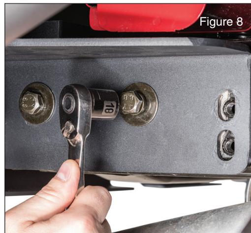
*It may be necessary to hold the plate in place with one hand while threading the bolts with another. (FIG8) Snug but do not tighten the bolts with a 18mm socket.*
