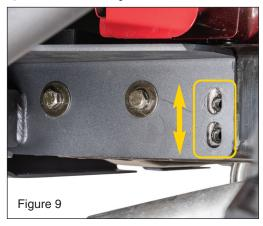
Adjust the bumper to the desired alignment. (FIG9) Then, install the M10 bolts, lock washer and flat washer in the smaller holes closer to the front of the vehicle and tighten the two M10 bolts with a 16mm socket and ratchet. Torque
