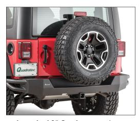
and standard 2" Quadratec receiver hitch (#12015.1000) as shown above.
