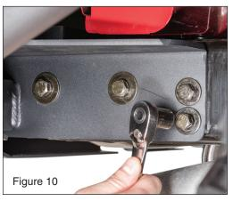
M10 Bolts to 37 ft lbs. (FIG10) Fully tighten the larger M12 bolts at this time with a 18mm socket. Torque M12 Bolts to 66 ft lbs.
