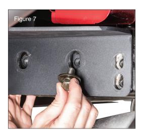
Align the holes in the bumper with the holes in the frame rails and the nut plates. Thread the 12mm bolts with lock washer and flat washer into the nut plates inside the frame. (FIG7)
