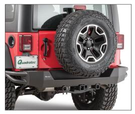
Bumper install is now complete. The ORC Rear Bumper is designed to be compatible with the VersaHitch® (#12015.1002)
