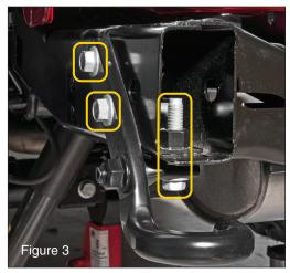
If equipped, remove the three bolts attaching the original recovery hook using a 18mm socket. (FIG3) Recovery hook will not be reused with the new rear bumper.
