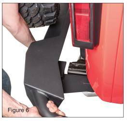
person, and with the tailgate partially open lift the bumper and gently rest it on the frame rails of the vehicle. (FIG6)
