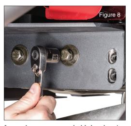
It may be necessary to hold the plate in place with one hand while threading the bolts with another. (FIG8) Snug but do not tighten the bolts with a 18mm socket.
