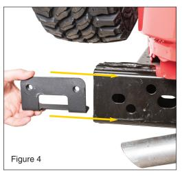
Insert the provided nut plates inside of the frame rails as shown (FIG4).
