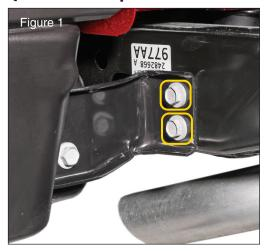
Put on safety glasses. Open the tailgate and swing it & the spare tire out of the way. Remove the four M10 bolts (2 per side) holding the rear bumper brackets to frame using a 16mm socket. (FIG1)
