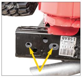
Align the threaded holes in the nut plates with the holes in the frame rail. (FIG5) Then, with assistance of another
