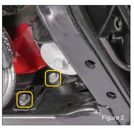
Remove the four M10 bolts holding the rear bumper support brackets to the frame using a 16mm socket. (see FIG2) Remove bumper from vehicle.
