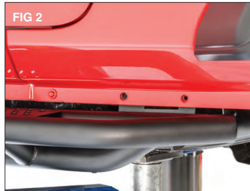
Starting at the front of the vehicle position the mounting tabs of the rock rails behind the pinch weld and align the holes with the factory pinch weld holes as shown. (FIG 2)
