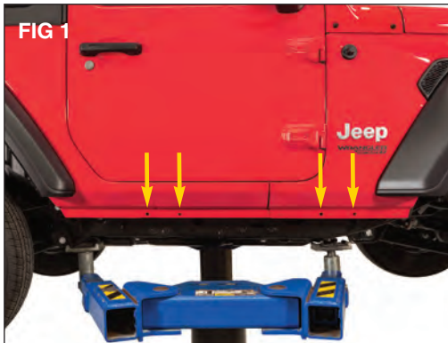
Put on safety glasses. Locate the 4 holes along the factory pinch weld of your vehicle as show in picture. (FIG 1)
