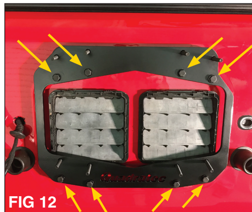
[FIGS 11 & 12] Tighten the 8 bolts to 13ft lbs.
