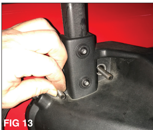
Thread in the 4 lower bolts, make sure the upper bolts are aligned in the rear plate before snugging bolts.
