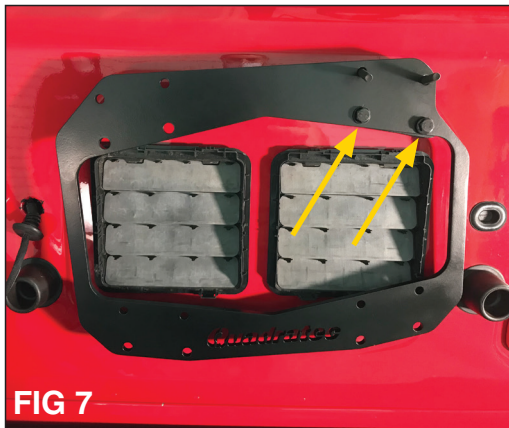
Start the 2 bolts in the tailgate so it holds the plate on the Jeep but do not tighten at this time. [FIG 7]
