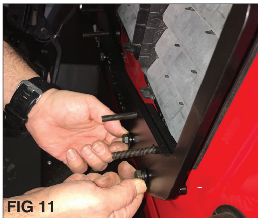
Thread in the 4 lower bolts, make sure the upper bolts are aligned in the rear plate before snugging bolts.
