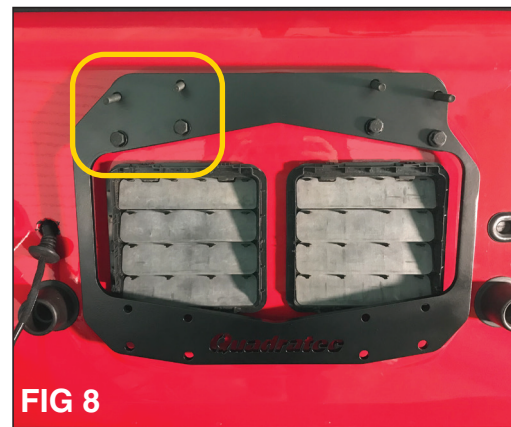
Repeat Steps 4 and 5 on the left side, again do not tighten at this time. [FIG 8]
