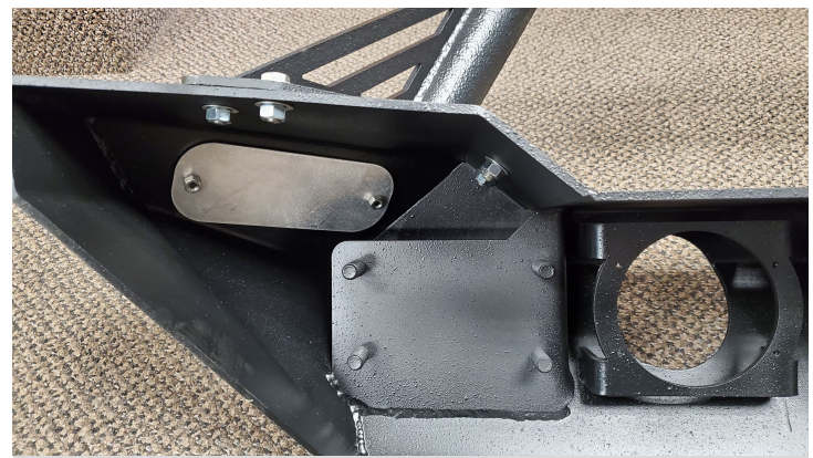
Detail 15: Accent plate & bull bar installed
