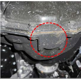
If the Differential does not have a drain plug the RS62116 will NOT fit on your application.
