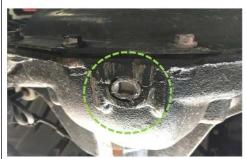
If the Differential has the drain plug the RS62116 will fit on your application.
