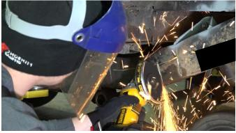
Once you've cut the body mount bracket free, remove the body mount bushing as it will be used during the replacement install.
