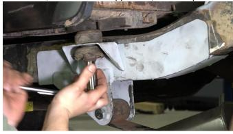
C-clamp or tack weld the part into place to prevent it from moving later.
