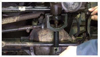
Using a Pitman arm puller, drop the Pitman arm and drop the steering box.
