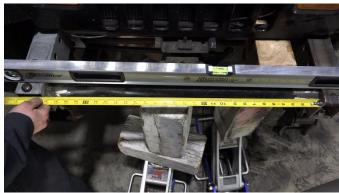
Take note of any difficulties and cut away any obstructions. The part may fit snugly and require force. If you have to bend the front cross member to fit the part into place, you may need to remove very small increments of material from the frame rail until it is flush. NOTE: Removing too much metal will make the gap size too large to fill with weld! Our part provides more material than what is needed for the install, per these instructions.
