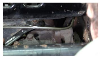
Using an 18mm wrench, disconnect the power steering tubes.
