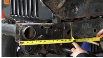
NOTE: The following steps require accurate measurements in order to allow correct amounts of weld-able frame.
