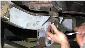
C-clamp or tack weld the part into place to prevent it from moving later.
