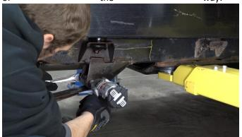
Using a 16mm socket, remove the body mount bolt from the bushing.
