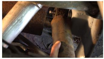
Reassemble the lower strut bolt and shock.
