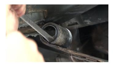
Depending on the exhaust routing, it may need to be removed or loosened to allow freedom of access.
