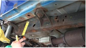
Mark down 1.5 inches from the top of the frame rail, on the inside and outside. You will do this from the front most body mount bracket to the bend at
