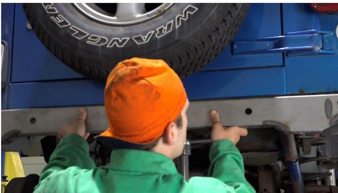
Ensure the two body mount bushing holes in the part line up with the body mount holes in the vehicle's body.
