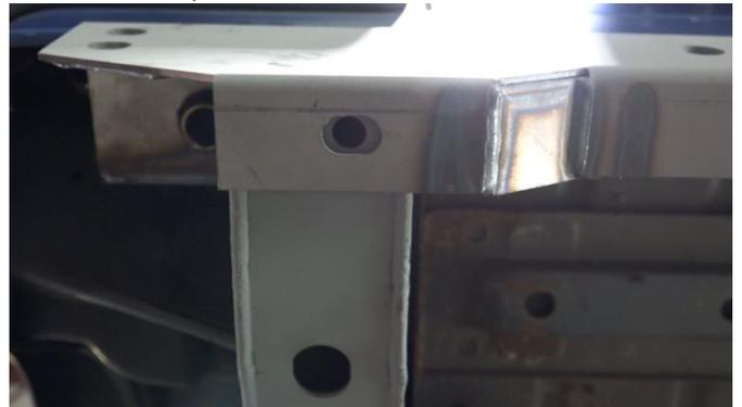
We recommend the Rear Cross Member be level. Note: Any frame deformations may result in the part sitting at an angle.
