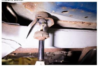
With a hydraulic jack and block, push up on the body of the vehicle, near the center, enough so that you can pull the body mount bushing out of its bracket.
