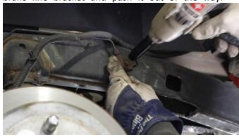
With a 5/8 socket, remove the 2 bolts from each track bar bracket and push it down and out of the way.
