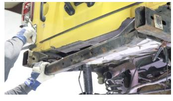
proper welding procedures begin welding the part onto the frame rails.
