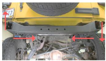
NOTE: WHEN THE REAR CROSSMEMBER IS REMOVED, THE FRAME RAILS WILL SHIFT. PRIOR TO THIS, TAKE AN OUTSIDE MEASUREMENT OF THE DRIVER FRAME RAIL TO THE PASSENGER RAIL, TO ENSURE THE INSTALLATION POSITION REMAINS CONSISTENT
