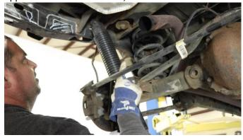
Just above both the coil spring buckets and the body mount crossmember is a wiring harness secured by body clips. Remove the clips with a body clip remover tool and push the harness out and away.
