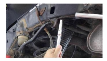
With an 18mm and 16mm sockets, remove the upper and lower shock bolts, and remove the shock.
