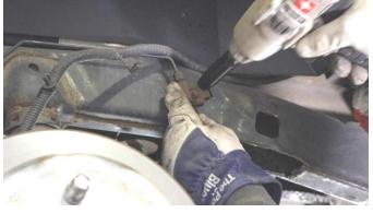
With a 5/8 socket, remove the 2 bolts from each sway bar bracket, and press it down and out of the way.
