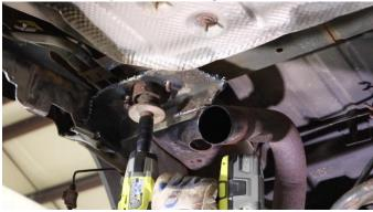
With a 16mm and 18mm socket, remove the body mount bolt, and continue cutting while avoiding damage to the body mount bushing.
