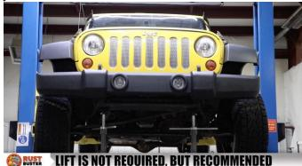
Remove your rear wheels, any inner fender liners, and any factory or aftermarket accessories that would pose as a fire hazard or prevent access to the work area.
