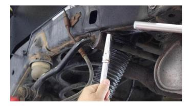
With an 18mm and 16mm sockets, remove the upper and lower shock bolts, and remove the shock.
