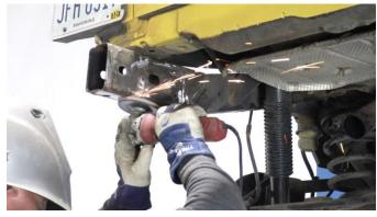
Hold the part up to the frame by roughly lining up the hole locations. Mark your intended cut line, removing as much rust as possible, while retaining a safe and weld-able margin.
