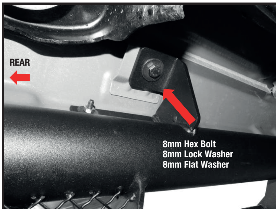
Driver/left side rear welded Bracket attached to inner floor panel
