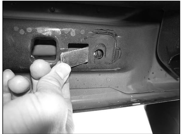
(Figure 6) Slide Nut Plate into channel
