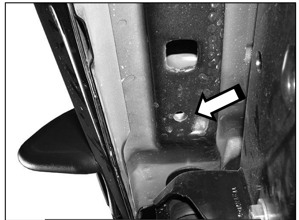
(Figure 8) Closed floor channel with factory 8mm threaded hole
