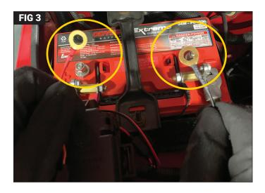
Locate your positive and negative fairlead wires. Connect the positive and negative wires directly to your positive and negative battery terminals. (FIG 3) **NOTE**: After the positive and negative connecters are connected to the battery the fairlead light will illuminate. After this step the Res-Q fairlead light bracket can be turned "On" and "Off" with the remote control included in the kit. Additionally, the remote will be used to change the color from "White" to "Amber" color.
