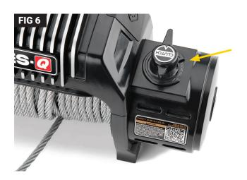
Once the trigger wire is connected to your winch, turn your winch "ON" and with the winch in free spool action the "In" or "Out" function of the winch to ensure the trigger wire functions properly. (FIG 6)
