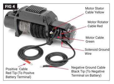
After securing the Res-Q Fairlead Light Control Module, continue to follow the "WHITE" trigger wire back to the winch motor area. The module is equipped to automatically turn on the LED Fairlead Light when the winch is activated. The trigger wire is to be connected to the "Motor Rotator Cable RED" located on the back side of the winch's motor. (FIG 4)
