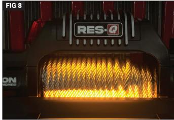
The Res-Q fairlead light will turn on for 15 seconds after the winch trigger wire is charged with 12v. The Fairlead light will illuminate with the last color that the module turned off with. The color can be changed by turning on the Res-Q Fairlead light with the remote and changing the color. Then turning off the fairlead light will save the alternate color as the trigger wire illumination color. (FIG 7 & FIG 8) Installation is now complete.
