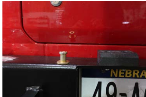
(Striker nut installed)
