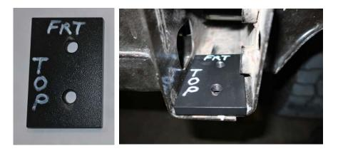
4. Set top lip of bumper on frame. Slide 2x 1-1/2" x 5/8" x 3-1/4" blocks with 2 holes between frame and lower lip of bumper. Make sure wiring is between bumper and block and will not get pinched. Use 2 factory bolts from tow hook on driver side. Use 2-1/2" x 3" full thread bolts with 2x 1/2" SAE flat washers on passenger side 18MM wrench on factory bolt using <sup>3</sup>/<sub>4</sub>" wrench on <sup>1</sup>/<sub>2</sub>" x 3" bolts. Do not tighten fully.
