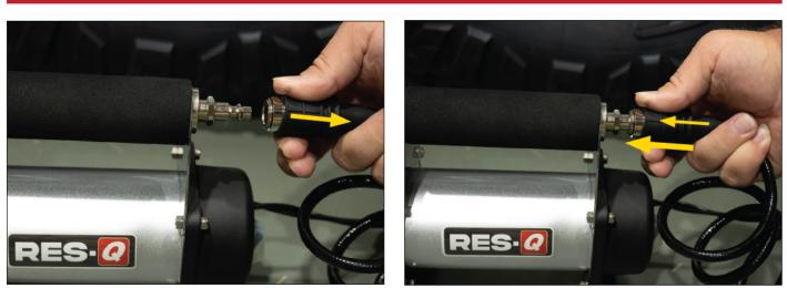
Put on safety glasses. Attach the ¼" quick connect coupler on the coiled hose to the ¼" quick connect stud on the air compressor by pulling the retaining ring under the rubber covering back. Slide the fittings together firmly. While holding the fittings together, slide the retaining ring closed toward the compressor to lock.
