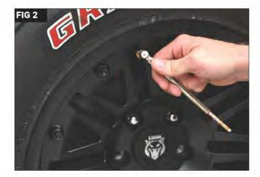
Put on Safety Glasses. Remove valve stem cap from the valve stem and deflate a tire to your desired air pressure using a Tire Guage. This will be the pressure the Res-Q Automatic Tire Deflator will be set to. (FIG 2)
