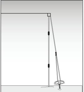
Awnings can have the screw positioned at the base of the leg to minimise trip hazards with extending guy ropes
