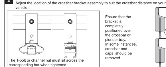
Ensure that the bracket is completely positioned over the crossbar or pioneer tray. In some instances, crossbar end caps should be removed.
