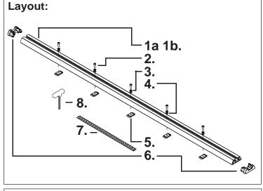
Install all security screws using spring washers, flat washers and channel nuts. Finger tighten.
