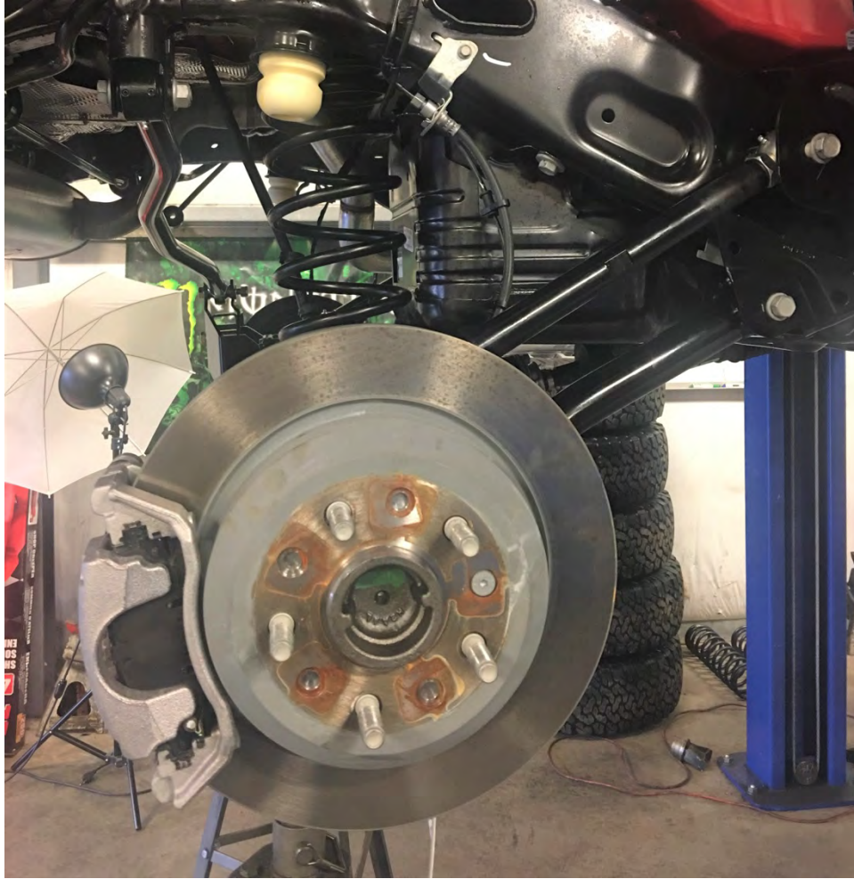
Rear Uppers and Rear Loweres Installed in the Vehicle
