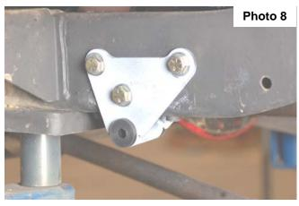
12. Reverse the springs and install what was the rear part of the leaf springs in the front mount using the supplied 9/16" x 4 1/2" bolts, nuts and washers. Only slightly tighten at this time. Raise rear of the leaf spring up to meet the new rear bracket. **Note:** On the small eye of the spring, remove bushings and install one shim behind each bushing and replace. **See Photo 9 & 10.**
