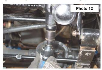
move the pitman arm. Inspect the shaft splines for excessive wear, repair if needed. Retain hardware for reuse.
