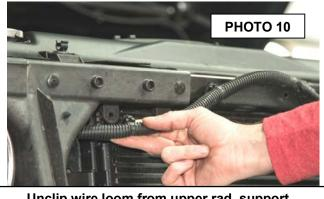
Unclip wire loom from upper rad. support.
