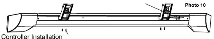
12. The controller mounting will be located near the center of the vehicle on the passenger side of the vehicle. Install the controller assembly with two (2) supplied M8x20mm hex head bolts, large 8mm flat washer, and 8mm spring washer. Tighten with a 13mm wrench. **See Photo 11.**
