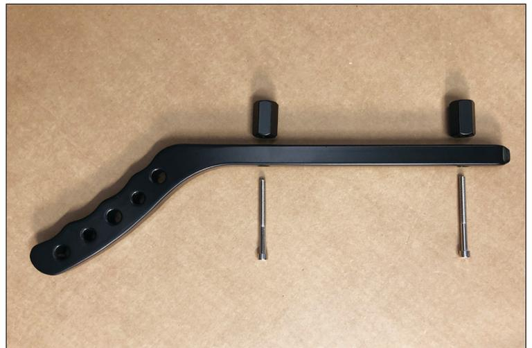
3. Insert Allen head bolt through the handle and then through the hex spacer into roll bar. **DO NOT** Overtighten the bolts or use power tools to tighten, it could cause the threads to be striped or bolt to break. When tightening alternate between to the two Allen head bolts to assure the handle seats flat to the roll bar.
