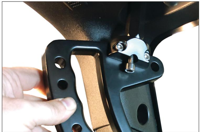
6. Now tighten bolts in an alternating pattern to avoid components from binding up. DO NOT use power tools. Tighten the two bolts snug but do not over tighten to avoid stripping the threads or breaking the bolt.
