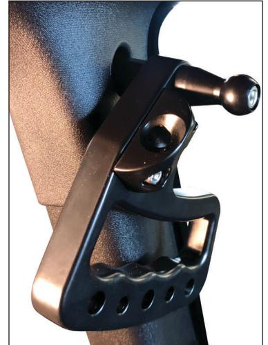
8. Now take the shorter bolt insert into the handle and then the hex spacer while rotating the handle into position. This can be a little tricky to align so take your time to avoid cross threading.
