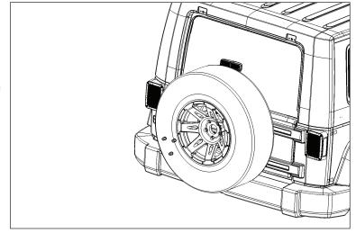
2. Place Mounting Plate onto spare tire carrier.
