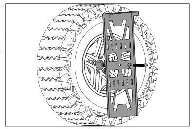
5. Torque M16 Bolt until Recovery Rack begins to slightly flex inward. Recovery Rack should not rotate compared to tire.
